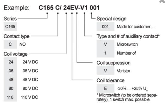
Type C contactors are NO contactors fitted with magnetic blowout. Here the NO contact functions as circuit-breaker within an open contact design.
